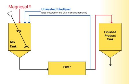
plant trial that involved the product, and a brief look at replacing the water-wash step with the company's magnesium silicate treatment.
